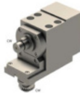
MSP-160 Polygon Milling ID Size: Ø16mm Output: 1:3 Max Tool Ø 58mm, High speed up to 18,000 RPM
