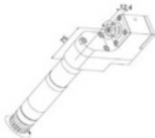
GSE-306-SE312 End Drill/Mill Collet Size: ER11 Output: 1:3 High Speed
