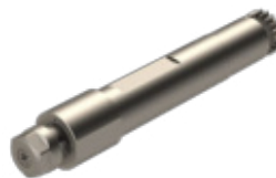
GSC-510-L-3X Cross Drill/Mill Collet Size: ER11 Output: 1:3 High speed up to 18,000 RPM
