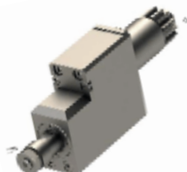
GSS610 Slitting Saw Saw ID: 10mm Output: 1:1 Max Tool \varnothing 40 mm Max Width 4.5mm
