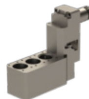
GSE1504 End Drill/Mill Bore Size: Ø31mm Output: 1:1 Holds 3 compatible spindles (GSC1110, GSC1110-4X, GSC1310-HP)
