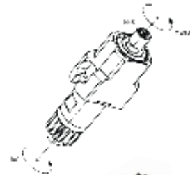
MSC507-HP Cross Drill/Mill Collet Size: ER11 Output: 1:1 Internal cooling Max 150 bar
