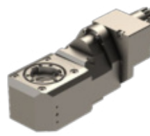
GSF-080 Polygon Milling Tool ID Size: Ø8mm Output: 1:1 Max Tool Ø 58mm Max Width 3mm
