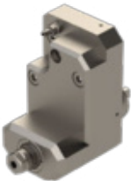
KSC-DEC-L-10x3-V Cross Drill/Mill Collet Size: ER11 Output: 1:3 External cooling, High speed up to 15,000 RPM, 6mm extended
