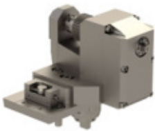
KSH432 Gear Hobbing ID Size: Ø10mm Output: 1:1 Coolant-thru Hobb OD: Ø32mm Hobb Width: 30mm Adjustable ±5°
