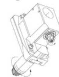
KSF-130-ER Polygon Milling Collet Size: ER11 Output: 1:1 Adjustable ±20°
