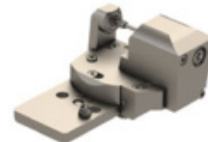
MSH210-080 Gear Hobbing ID Size: Ø8mm Output: 1:0.846 Coolant-thru Hobb OD: Ø24mm Hobb Width: 16mm Adjustable \pm 10^\circ
