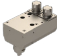
KSC313 Cross Drill/Mill Collet Size: ER20 Output: 1:1 External cooling, Requires Y-Axis
