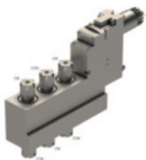
BSA-2010 Angled Drill/Mill Collet Size: ER16 Output: 1:1 Adjustable 0-21° Interferes with adjacent tooling position
