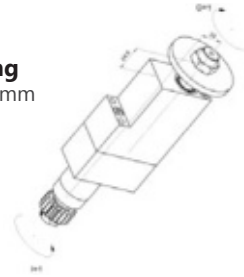
GDF-1207-L Tool Holder Tool Size: Ø19.05mm (3/4in) 4 Tool Positions A 2 20VII
