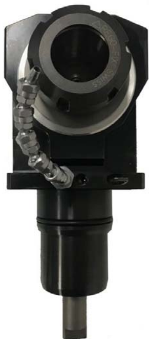
DECA system mounted in rotary tool holder. Straight nozzle ID:3 mm & L:10 mm
