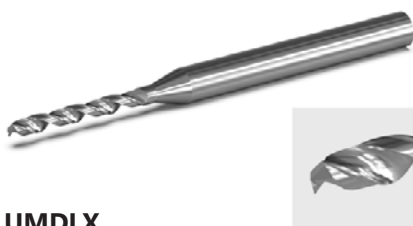
UMDLX ... Point relief: 4 facet, 130° With x-point for self-centering
